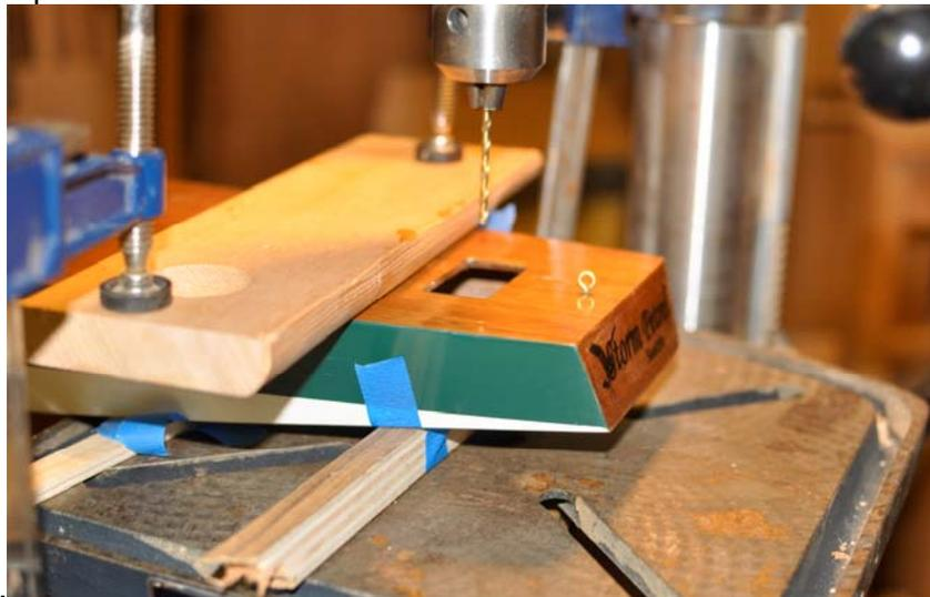
The 1/8 inch drill in the chuck enables accurate location of the drill press centered on the existing hole. The shims are different thickness and were located fore-and-aft to make
