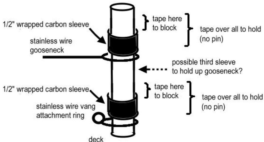
Note: 1/4" of the barrel of a BIC pen does just as well as a carbon sleeve here.
