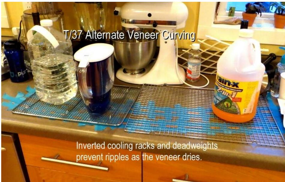
Inverted cooling racks and deadweights prevent ripples as the veneer dries.
