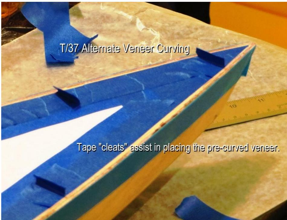
Tape "cleats" assist in placing the pre-curved veneer.
