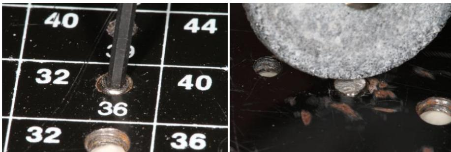
Center hole of fittings need to be enlarged to slightly less than 1/4". I used a size B twist drill. Hole for set screw is drilled with a twist drill that matches (#32?) a 6x32 tap. Holes for cotter pin and Spectra are drilled with a 1/16" twist drill. A fine file is used to make a groove for the cotter pin to be bent over inside the lumen of the aluminum fitting and also for clearance inside for the Spectra.
