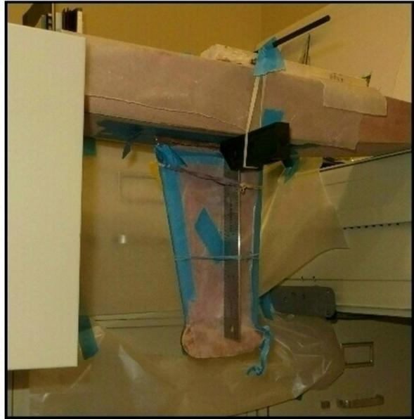
Keel web is held perpendicular to the bottom of the hull between two small carpenter squares. The squares are held against the web and against the hull by rubber bands. No "sighting" or judgement calls are required. Hull does not have to be maintained level. **Note that the web has been pre-shaped, but the keel bulb has not yet been attached.**
